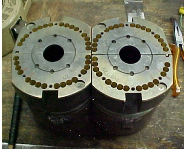
Figure 3 – Diffuser exits implemented on a mold
